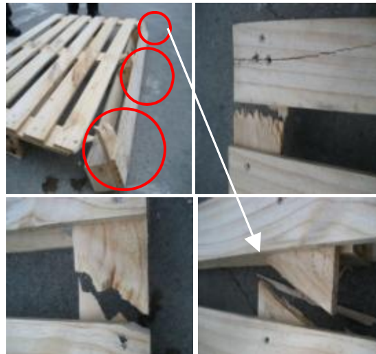
wooden pallet with broken stringer
