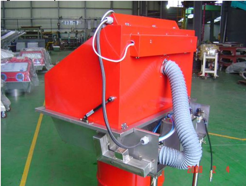
Figure 3: Rear of parts washer
