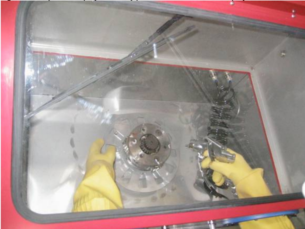
Figure 4: Low pressure spray and rotary plate. Not visible is second spray nozzle with brush on end.
